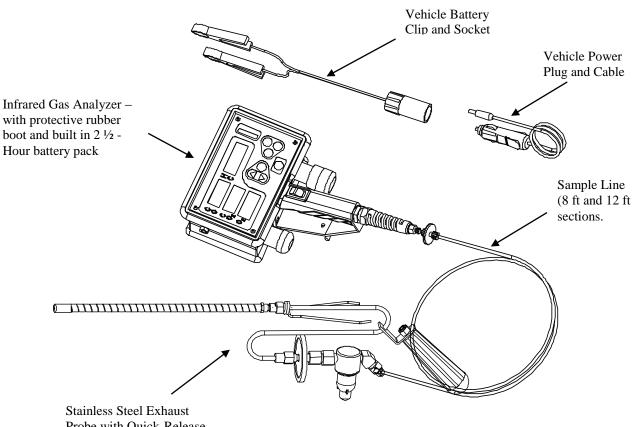
Stainless Steel Exhaust Probe with Quick-Release Flexible Tip and Built In Water Trap.
