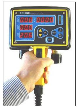
A 'Lo' message on the O2 display after the analyzer is Zeroed means that the O2 sensor is becoming too weak to provide reliable operation, and it should be replaced. The O2 sensor is located on the analyzer case at the left side of the handle is an operator serviceable item – as it is gradually consumed during operation and is intended to be replaced in the field when it expires after 12-18 months of service.
