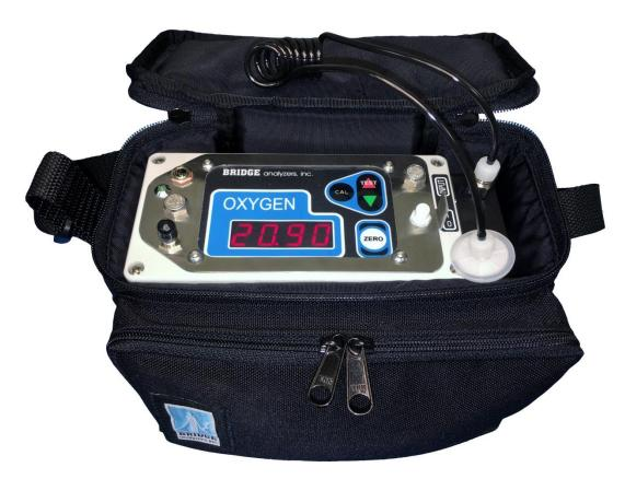
Down to 0.001% for Residual O2 and Up to 100% for Enhanced Oxygen
